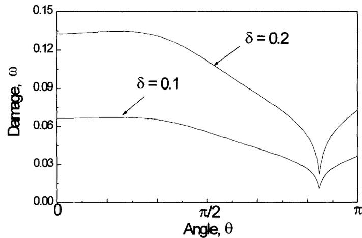
Fig. 9. The angular distribution of damage with  $\delta = 0.1, 0.2$ , while  $n = 4.64$ ,  $\mu = 1.47$ ,  $k = 4.94$ .
