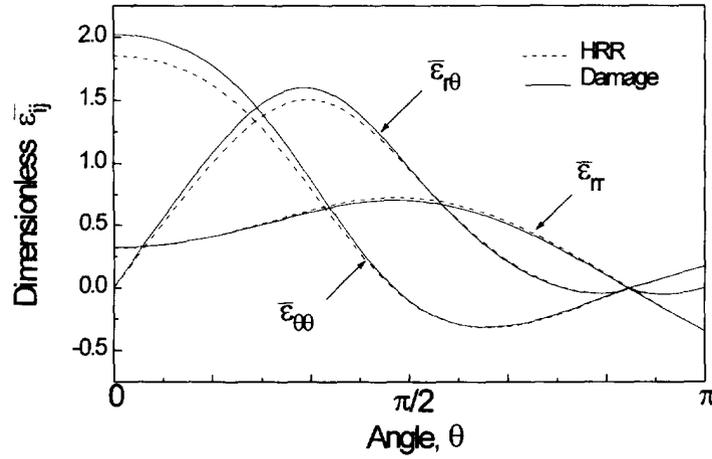
Fig. 8. The angular distribution of dimensionless strains for HRR field and damaged field with  $\delta = 0.2$ , while  $n = 4.64$ ,  $\mu = 1.47$ ,  $k = 4.94$ .
