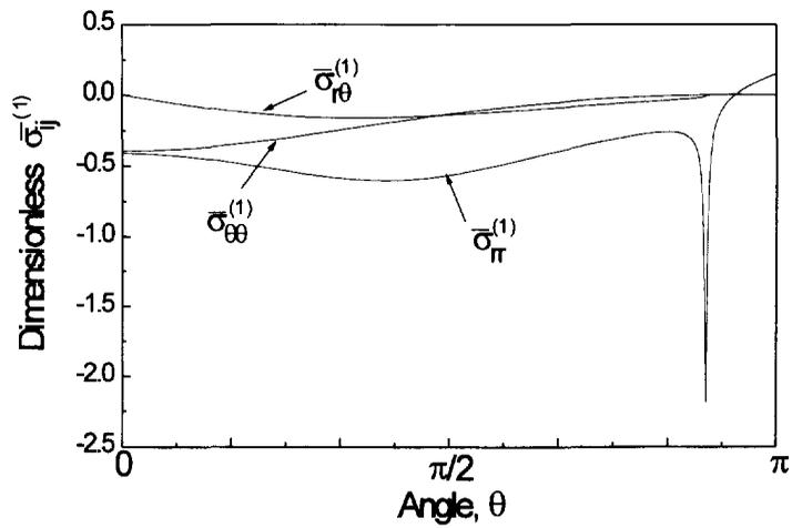
Fig. 3. The angular distribution of the first order perturbation stress field  $\bar{\sigma}_{ij}^{(1)}(\theta)$  with  $n = 3.1$ ,  $\mu = 1.52$ ,  $k = 2.2$ .
