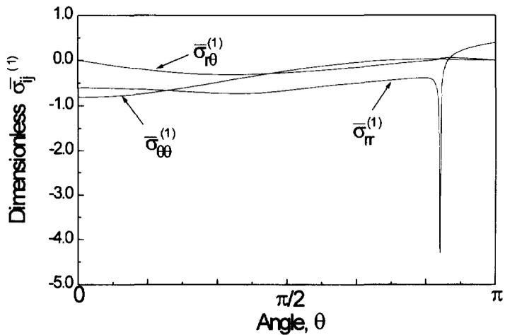
Fig. 4. The angular distribution of the first order perturbation stress field  $\bar{\sigma}_{ij}^{(1)}(\theta)$  with  $n = 5.5$ ,  $\mu = 1.52$ ,  $k = 2.2$ .
