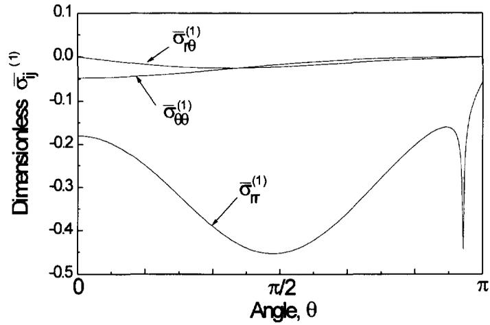
Fig. 2. The angular distribution of the first order perturbation stress field  $\bar{\sigma}_{ij}^{(1)}(\theta)$  with  $n = 1.5$ ,  $\mu = 1.52$ ,  $k = 2.2$ .
