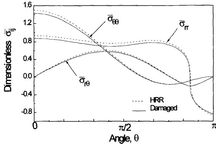
Fig. 5. The angular distribution of dimensionless stresses for HRR field and damaged field with  $\delta = 0.1$ , while  $n = 4.64$ ,  $\mu = 1.47$ ,  $k = 4.94$ .
