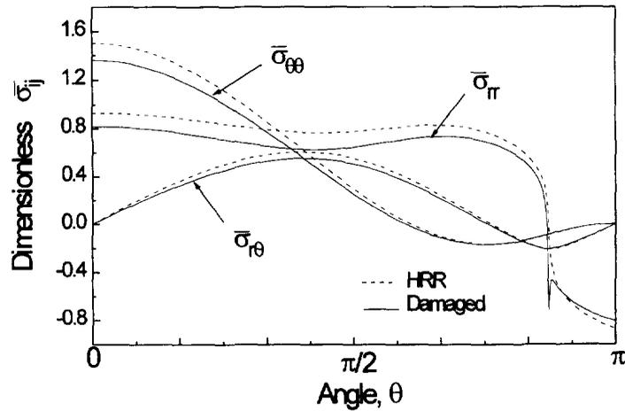
Fig. 6. The angular distribution of dimensionless stresses for HRR field and damaged field with  $\delta = 0.2$ , while  $n = 4.64$ ,  $\mu = 1.47$ ,  $k = 4.94$ .
