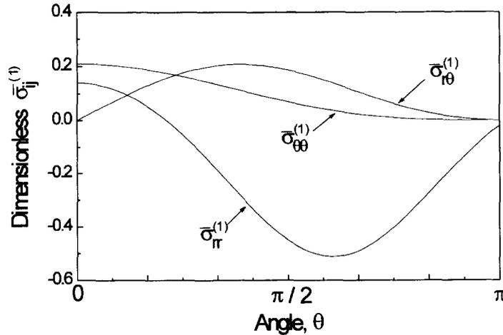
Fig. 1. The angular distribution of the first order perturbation stress field  $\bar{\sigma}_{ij}^{(1)}(\theta)$  with  $n = 0.8$ ,  $\mu = 1.52$ ,  $k = 2.2$ .
