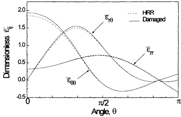
Fig. 7. The angular distribution of dimensionless strains for HRR field and damaged field with  $\delta = 0.1$ , while  $n = 4.64$ ,  $\mu = 1.47$ ,  $k = 4.94$ .
